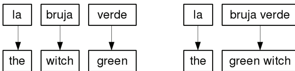
Figure 3. In the word-based translation on the left we see that the noun-adjective reordering into English is missed. On the right, the noun and adjective are translated as a single phrase and the correct ordering is modelled in the phrase-based translation.
